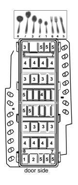
If the cutlery basket is equipped with two removable grids: insert the cutlery one by one into the slots, with the handles at the bottom. Position them so that they don't touch.
